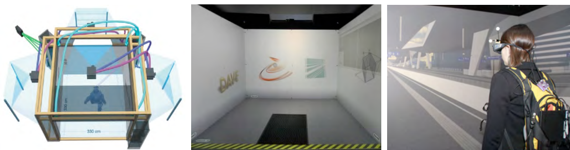
Figure 1. Immersive virtual environment DAVE and a test person equipped with eye tracking
