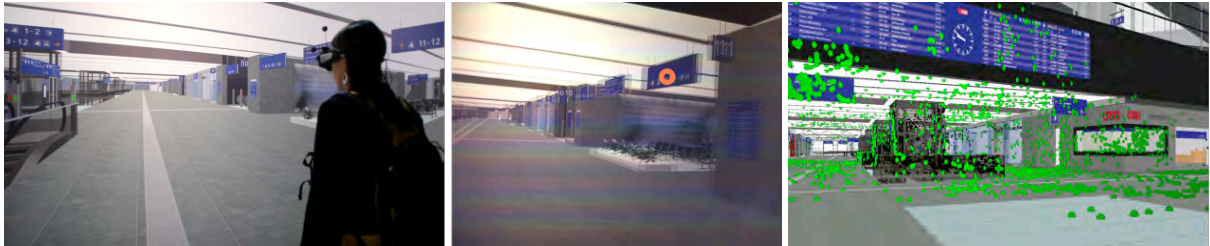
Figure 2. Test person in the virtual environment (left), eye tracking video frame with gaze point (center), visualization of attention (right)
